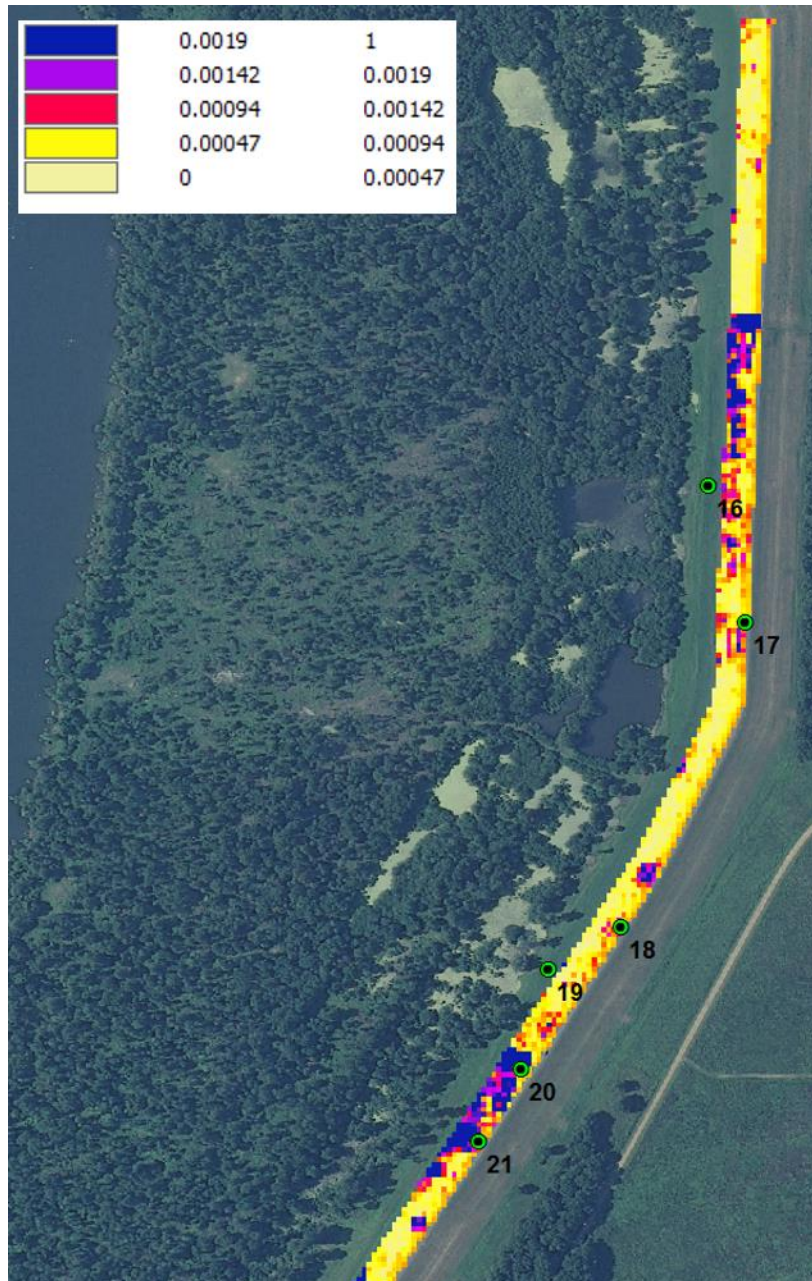
Figure 6.5 RX Anomaly detector classification output for active slides 20 – 21 at the time of UAVSAR image acquisition on 16 June 2009.
