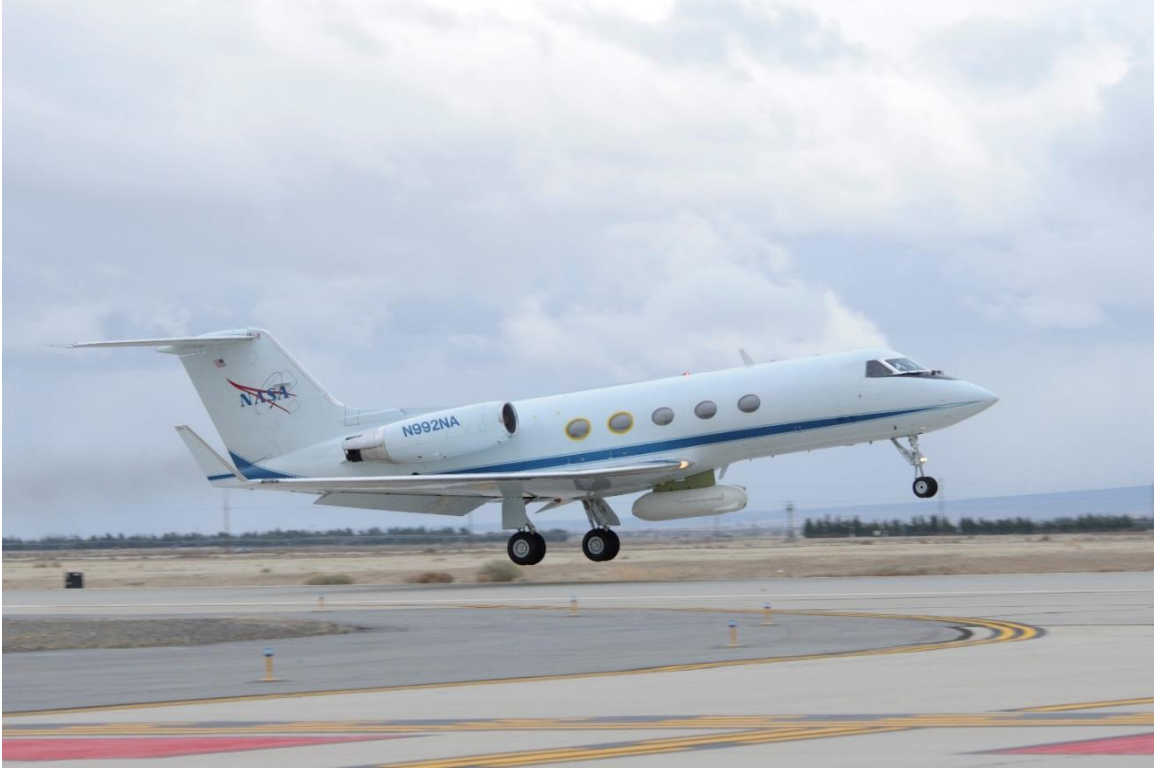
Figure 3.3 NASA Gulfstream III aircraft with a pod housing the UAVSAR
